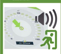
Press start in the center of the dial. The robot will beep for 15 seconds and start automatically.
