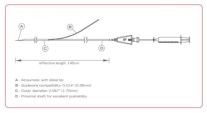
STENTYS® AC is indicated for the containment and aspiration of embolic material (thrombus/debris) while performing PTCA and/or stenting procedures, including in saphenous vein grafts.
