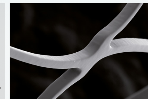
SEM of stent surface
